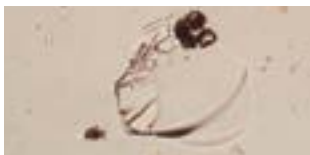
Beware of artefacts, e.g. this is a chip on the microscope slide
